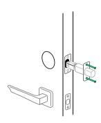
Remove your existing lock from your door, insert the provided latch, and secure it in place, ensuring the "Up" sign is pointing upwards.
